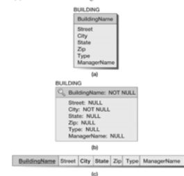
Figure 5.2 Transforming an Entity to a Table (a) BUILDING Entity; (b) BUILDING Table and (c) Alternative Table Diagram
