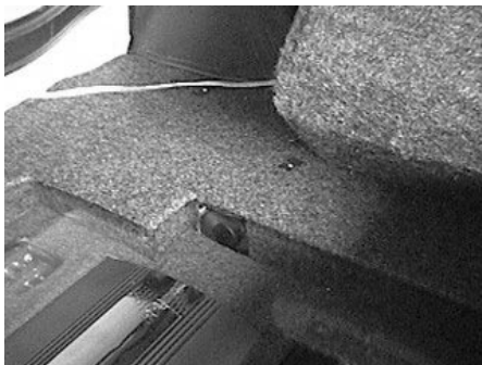
Figure 5: The cooling fan is running, and the Velcro that holds the subwoofer enclosure in place can be seen.
