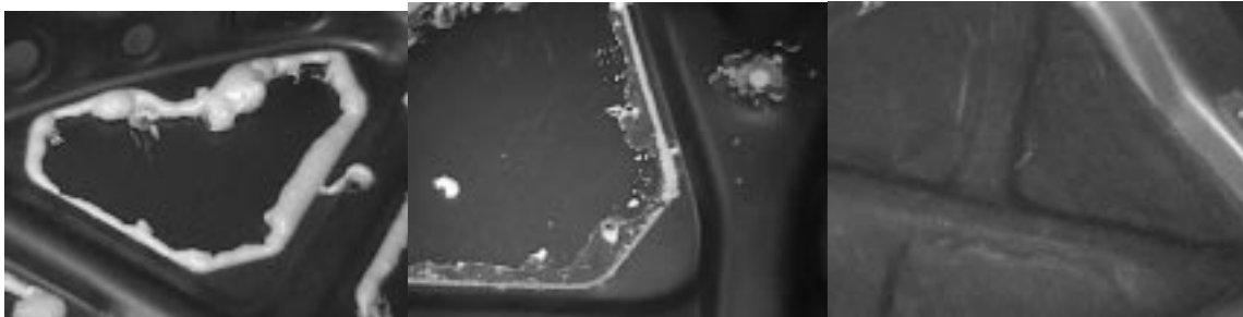
Figure 4: Steps taken when sound dampening the trunk lid.
