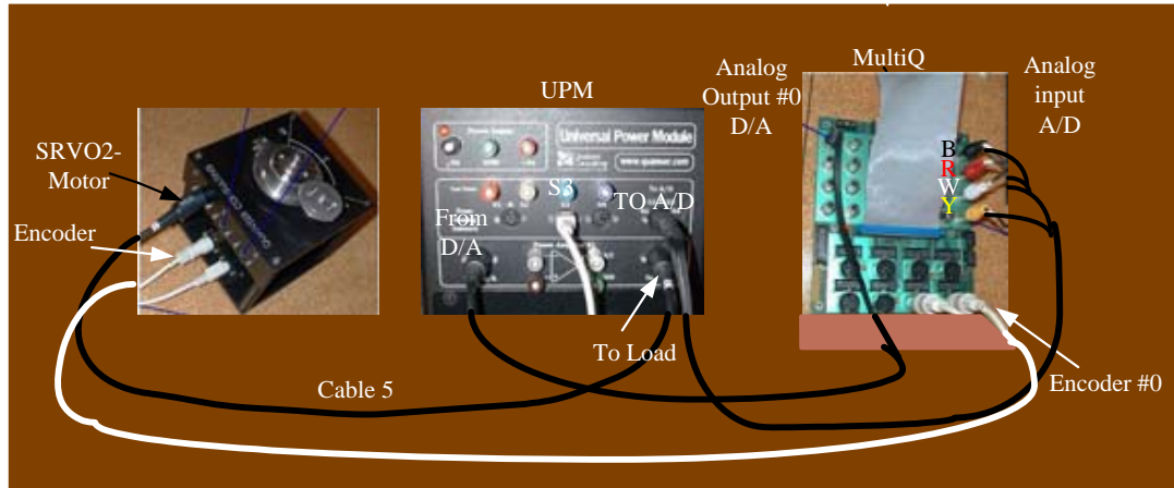
Figure 7.7 Wiring diagram for servo motor position control system.
